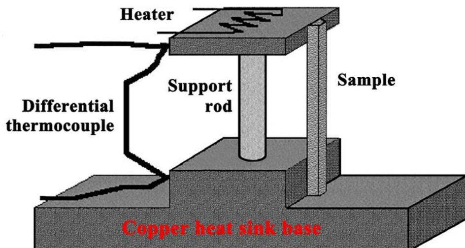
**Fig. 2.** Schematic illustration of the configuration of the parallel thermal conductance technique. The baseline was measured with the sample holder itself and then the sample was attached to perform the measurement of parallel thermal conductance in which the baseline was subtracted
