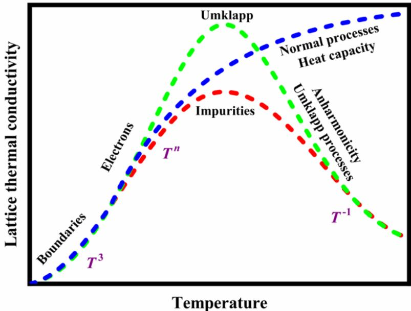
**Fig. 9.** Schematic illustration of the various mechanisms responsible for the temperature dependence of lattice thermal conductivity
