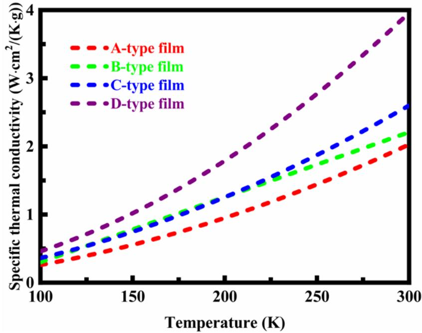
**Fig. 5.** Specific thermal conductivity of the carbon nanotube-based films at different temperatures. There exist significant differences in terms of structure, purity, and alignment between the films
