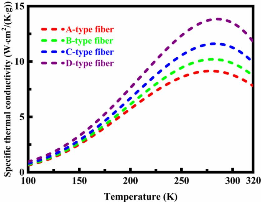
**Fig. 8.** Specific thermal conductivity of the carbon nanotube-based fibers at different temperatures. There exist significant differences in terms of structure, purity, and alignment between the carbon nanotube-based fibers
