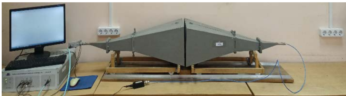
Fig. 6. The appearance of the measuring system when calibration before measuring of S_{21} values
