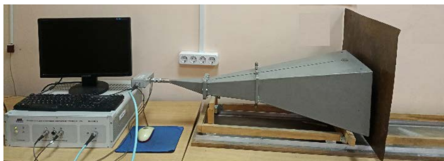
Fig. 3. The appearance of the measuring system when calibration before measuring of S_{11} values
