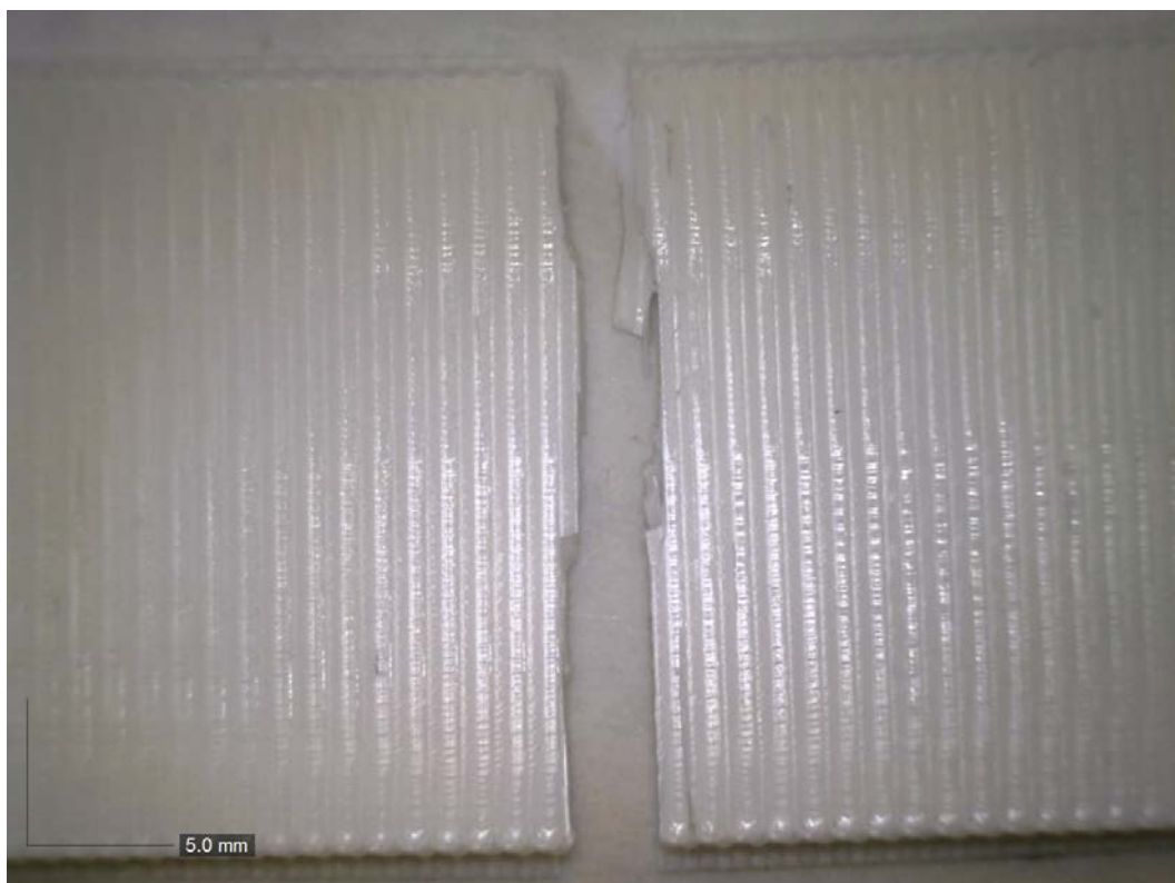
Fig. 6. Fracture surface of B5 sample made of PLA with double-weave (top view)
