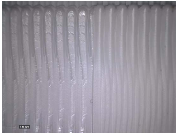
Fig. 2. Example of the two-layer weave of polymer threads in the right-to-left direction
