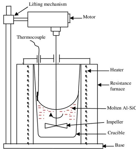
**Fig.1. Stir Casting Setup**
