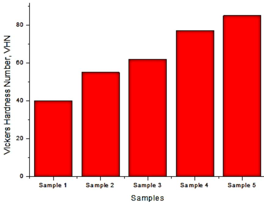
**Fig. 4.** Hardness test analysis of Al7075/Mica Powder
