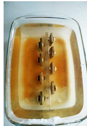
Fig. 2. Collected assemblies of pair samples in 5 % NaCl solution at 80 °C
