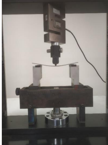
Fig. 3. Schematic of three-point bend test
