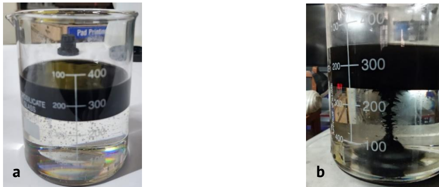
Fig. 1. (a) GO mixture with epoxy resin and (b) magnetic stirrer action of GO and resin mixture
