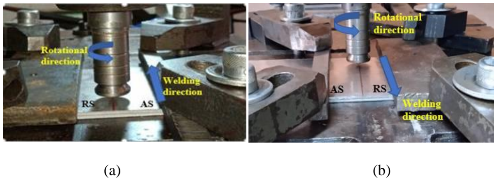
Fig. 3. Stir welded Lap joint: (a) configuration (A), (b) configuration (B)
