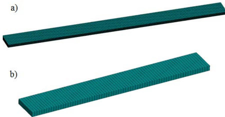
Fig. 3. Finite element models of a unidirectional composite material at the macro level. a) tensile test specimen; b) bend test specimen
