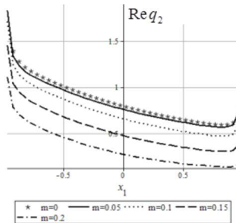
**Fig. 1.** Influence of porosity of a heterogeneous base on the distribution of the real part of normal contact pressure
