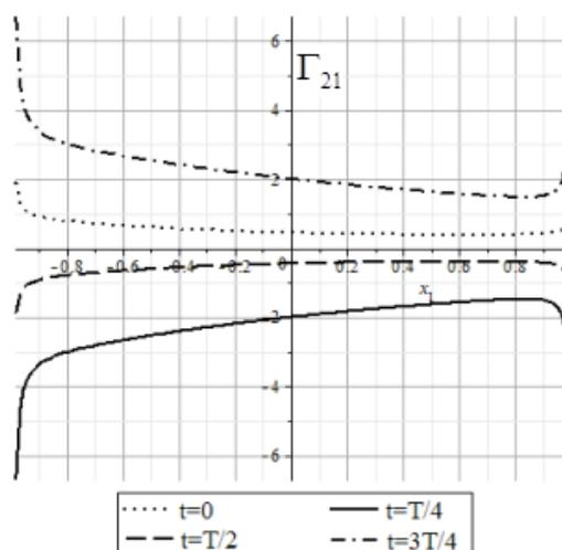
**Fig. 3.** Change in the tangential stresses during the vibration period  $T$
