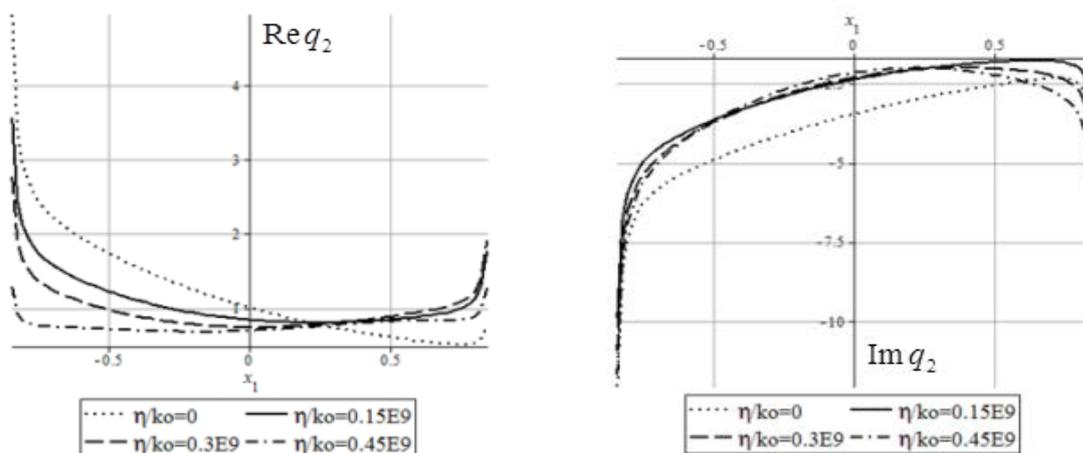
**Fig. 2.** The effect of fluid viscosity and permeability on the distribution of the real (left) part and imaginary (right) part of normal contact pressures
