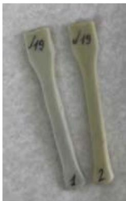
**Fig. 3.** Specimens 1 and 2 with the oil contents of 20 and 25 weight parts, respectively, for SIS VECTOR 4111NS
