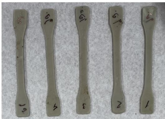
**Fig. 1.** Dumbbell-shaped specimens for testing
