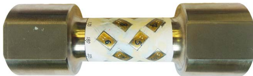
Fig. 5. Specimen with strain gauges before torsion testing (principal strains are located at an angle of 45^\circ to the axis of the specimen)
