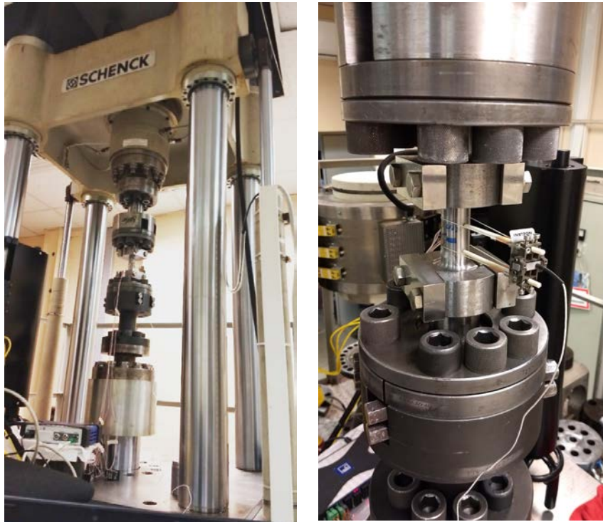
Fig. 3. Testing machine POZ 0909 manufactured by Schenck GmbH (Germany) with a control system BiSS (India), a maximum tensile/compressive load of 630 kN, and a maximum torque of 8 kNm
