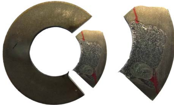
Fig. 4. Annular plates after etching and the SX texture
