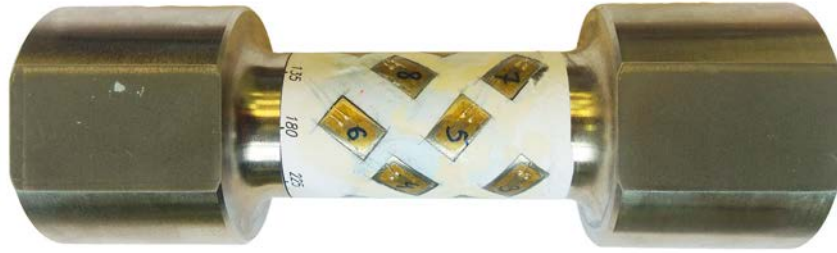
Fig. 5. Specimen with strain gauges before torsion testing (principal strains are located at an angle of 45° to the axis of the specimen)
