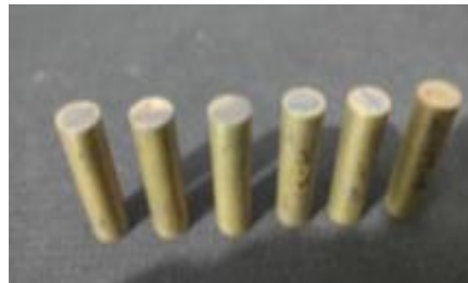
Fig. 4. Wear test specimen
