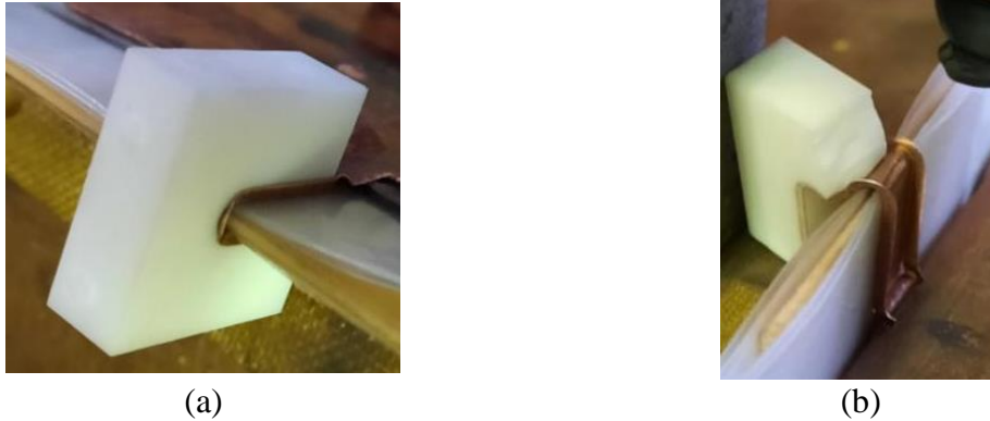
Fig. 4. Samples after testing: (a) the charging voltage is less than the threshold; (b) the charging voltage is above the threshold
