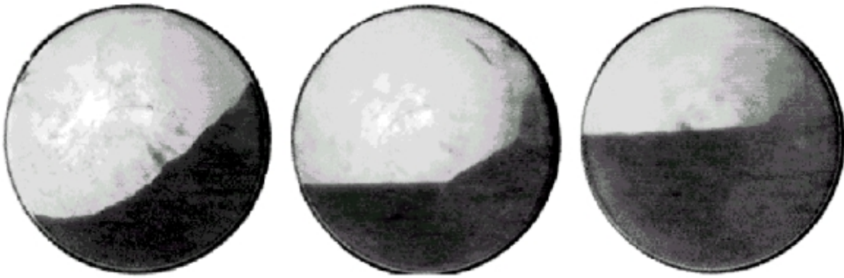
Fig.1. Behaviour of a cohesive powder in a rotating drum for three different angular speeds: \omega=10 rpm, \omega=45 rpm, \omega=100 rpm from left to right. The material is fluidized where the free surface is horizontal.
