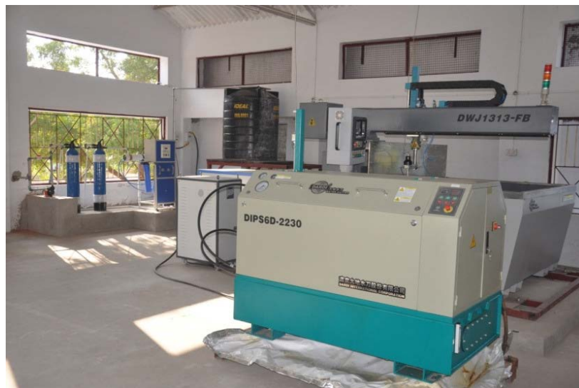
Fig. 2. Abrasive water jet machining setup
