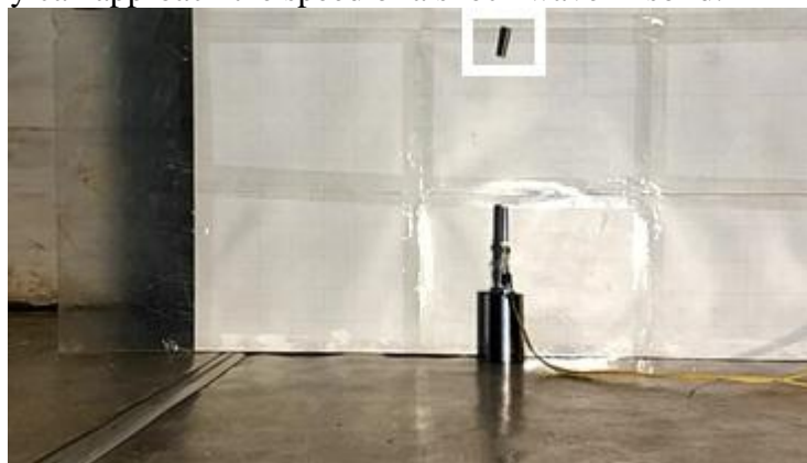
Fig. 4. Video snapshot showing a jump of a 30 g load as a result of burst-like shape memory strain recovery in 1.6g grams Cu-Al-Ni crystal. The initial speed of the crystal is 12 m/s. The launcher consists of a guide tube, an SMA crystal (inside the tube), and a heater
