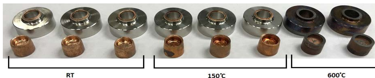
Fig. 8. The photos of the bimetallic samples after the rupture tests
