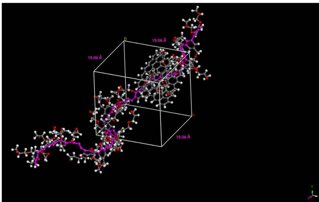
**Fig. 5.** The amorphous cell of Graphene Reinforced Epoxy
