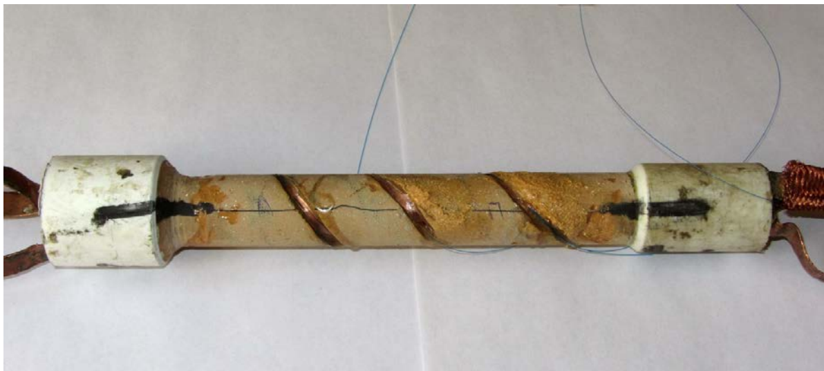
Fig. 7. Type II sample (winding is coated with a layer of epoxy resin with slots for placing the sensors)
