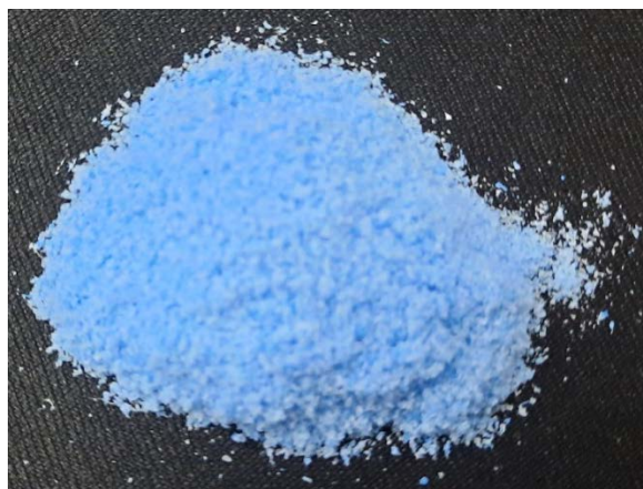
Fig. 1. Secondary polymer composition for rotational moulding RotoPolM115CB (RotoPol M115CB) after grinding on a mixer
