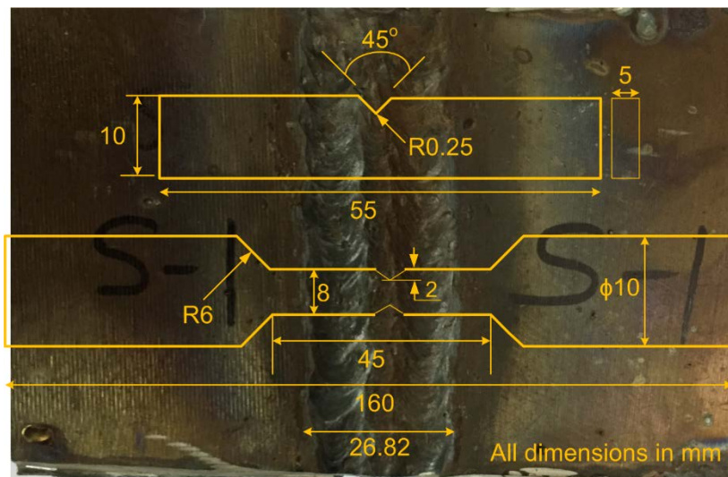
Fig. 3. Schematic of tensile and Charpy toughness specimen machined from the welded plate
