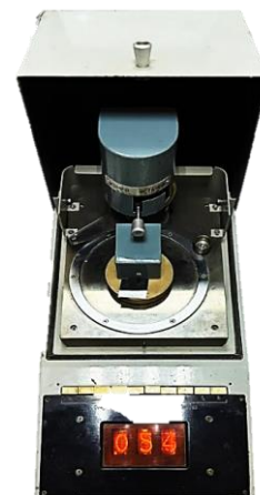
Fig. 9. External view of the measuring unit IUS-3 with an installed sample
