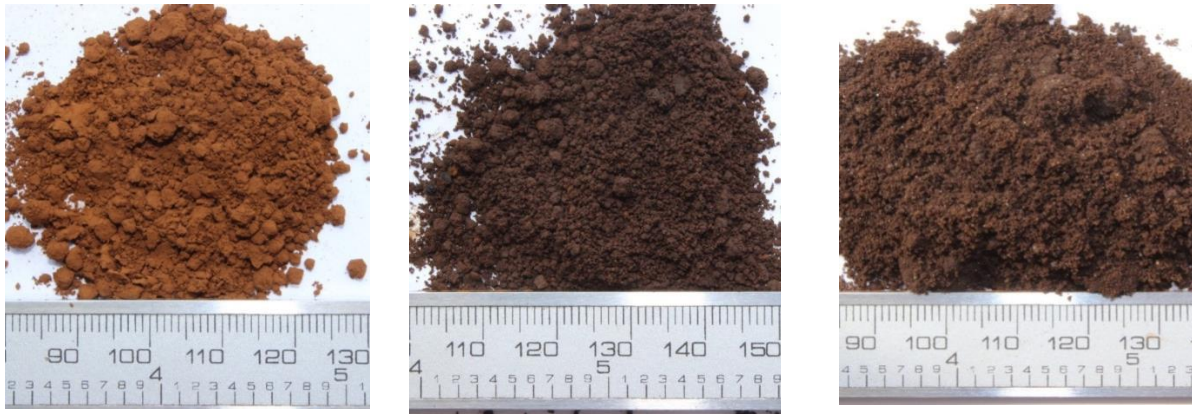
Fig. 1. Photograph of the appearance of various types of contaminants in the main gas
