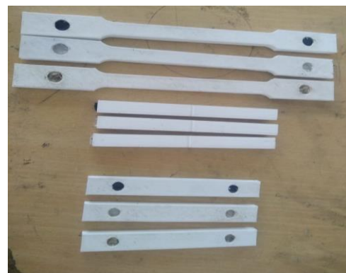
Fig. 3. Test samples after curing of fibre – epoxy resin in the ABS structure
