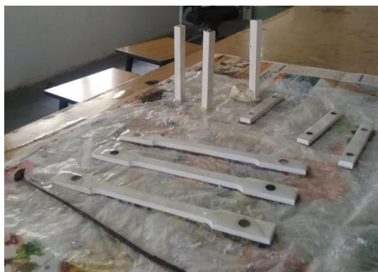
Fig. 2. The filling of fibre – epoxy mixture in the ABS structure
