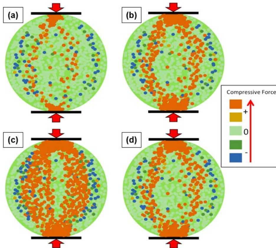
**Fig. 8.** The model of particle stress distribution in the bioplastic during the loading. Particles are colored according to the corresponding particle stresses. Light green represents a perfect structure, blue or green showing for low stress, and red color for high stress. The system to be investigated is represented by a visualization cell, in which all particles are enclosed and interacted. The top and bottom surface is subjected to a compression force in y-direction
