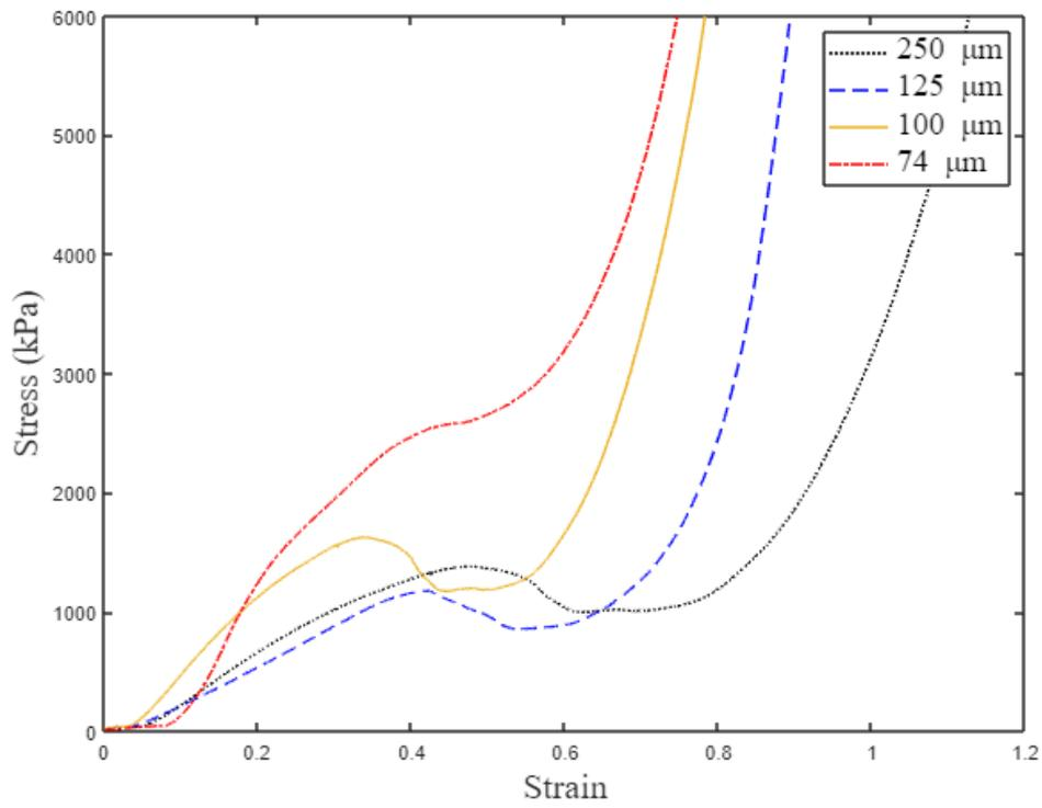
**Fig. 5.** Stress vs Strain of bioplastic samples
