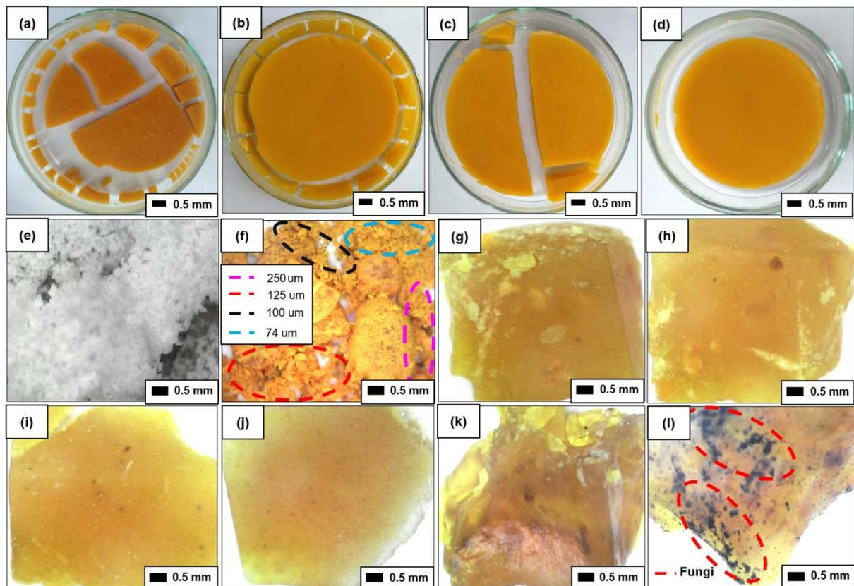
**Fig. 2.** Photograph image of cornstarch-based bioplastics with the addition various size turmeric (a) 250, (b) 125, (c) 100 and (d) 74 μm. Microscope images of (e) micro-sized cornstarch, (f) turmeric powder, (g-j) bioplastic prepared using turmeric with sizes of 250, 125, 100, 74 μm, respectively, (k) bioplastics after 6 days immersed in water and (l) fungi bioplastic after 4 weeks immersed in water
