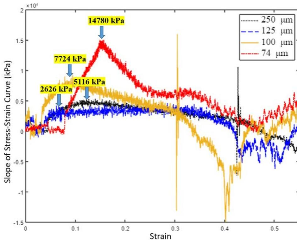
Fig. 7. Young's modulus vs Strain of bioplastic samples
