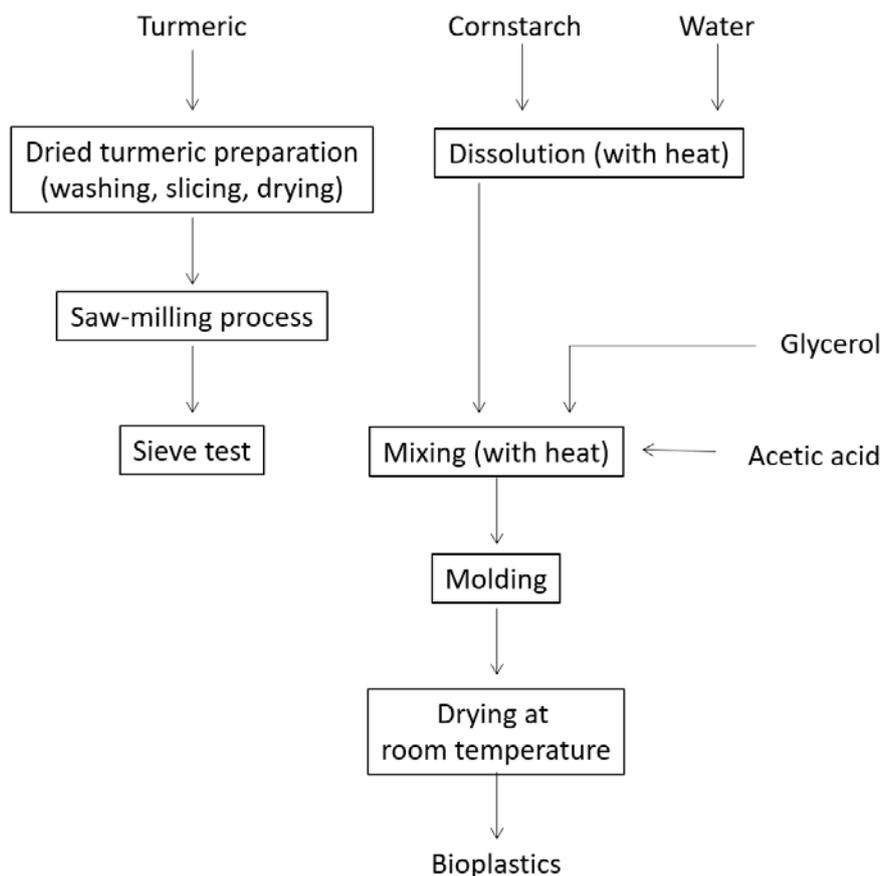
**Fig. 1.** Experimental procedure for the preparation of bioplastic
