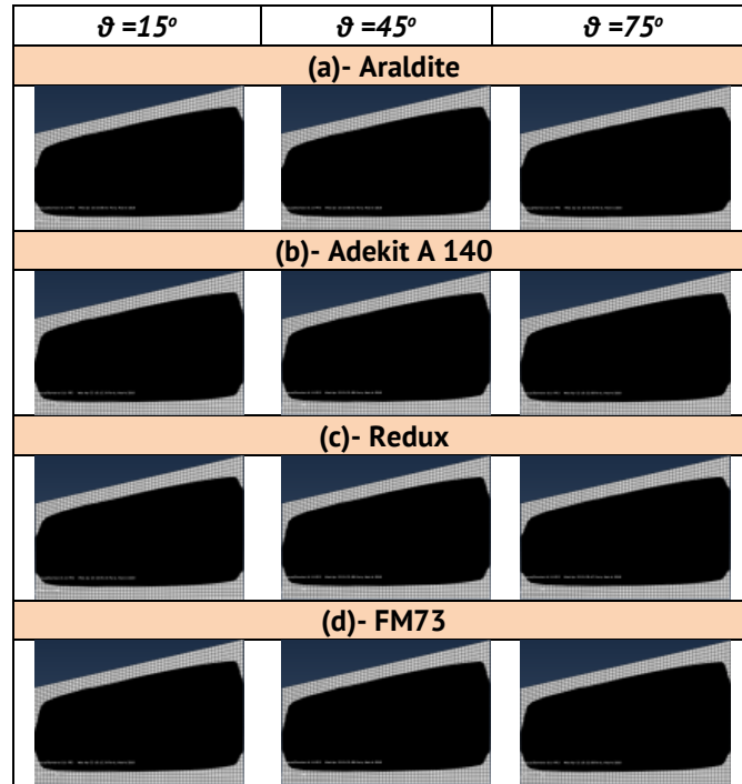
Fig. 9 Damaged area for a patch of trapezoidal shape and glue (a) Araldite, (b) Adekit A 140, (c) Redux and (d) FM73
