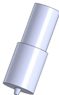
Fig. 1. Schematic drawing of the stirring tool
