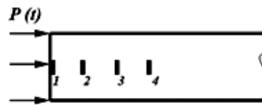
Fig. 2. Loading of snow solid by plane wave, 1-4 - position of sensors.
