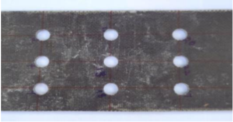
Fig. 3. Holes being laid over the finished sample.
