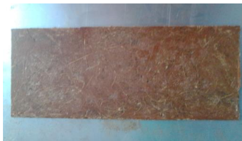
Fig. 5. Specimen of red mud filled Palmyra fruit fiber and Palmyra waste fiber.
