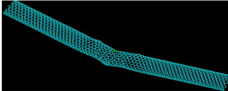
**Fig. 8.** The structure of carbon nanotube with simple heptagon topological defect.
