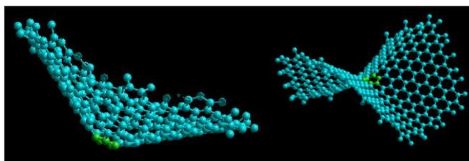
**Fig. 1.** Graphene layer fragment containing simple topological defect
