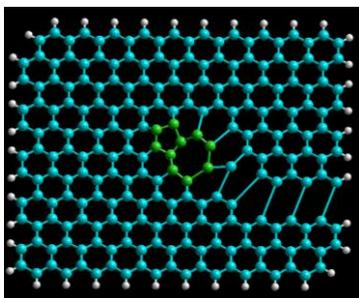
**Fig. 5.** 5-7 line defect.
