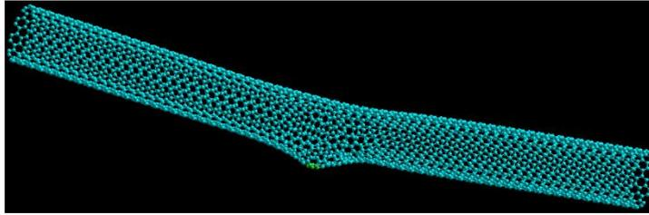
**Fig. 7.** The structure of carbon nanotube with simple pentagon topological defect.
