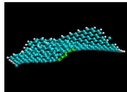
Nanotubes with simple penta- and heptagon topological defects were formed by twisting graphene sheet with corresponding defect into a tube. Then the tube is completed by connecting 10x10 carbon nanotube. As a result new carbon nanotubes depicted in Figs. 7 and 8 are formed.
