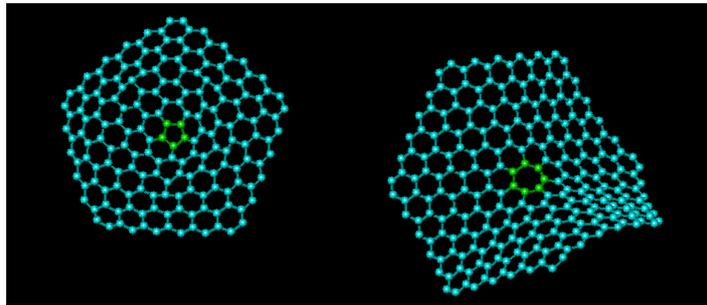
**Fig. 9.** Fragment of graphene layer with simple pentagon and heptagon topological defect.
