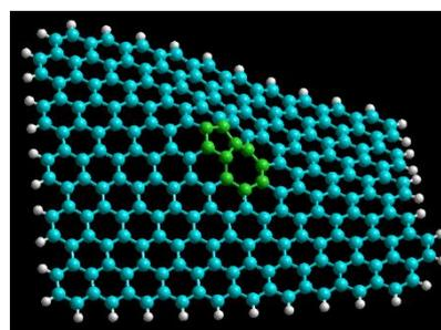
**Fig. 6.** 5-7 line defect after structure geometric optimization.
