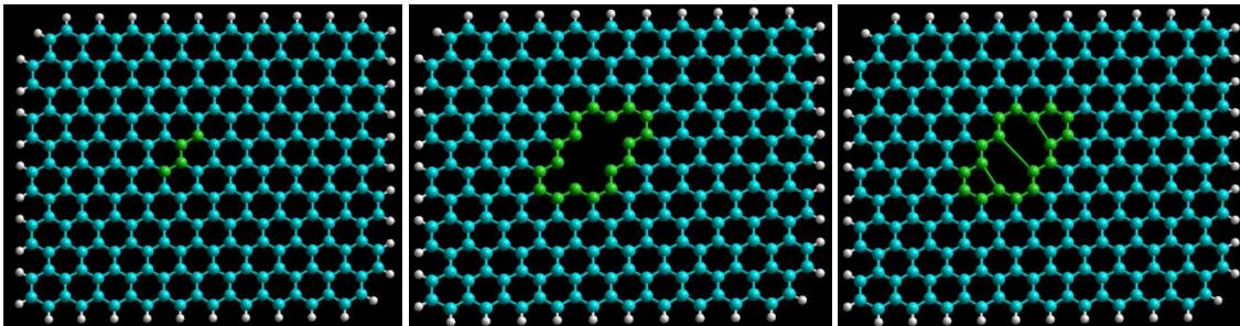
**Fig. 4.** a) Four atoms in graphene layer to be removed; b) Graphene layer after the removal of four atoms; c) Complex 5-7-7-5 spot defect formed in graphene layer.
