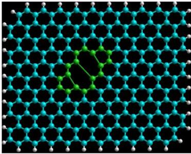
**Fig. 2.** 5-7-7-5 spot defect.
