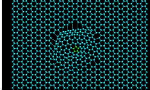
**Fig. 12.** Resulting graphene layer with defect.
