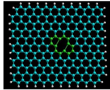
**Fig. 3.** 5-8-5 spot defect.
