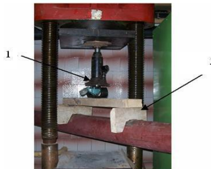
Fig. 1. Experimental assembly: 1 – thrustor, 2 – loading device.
