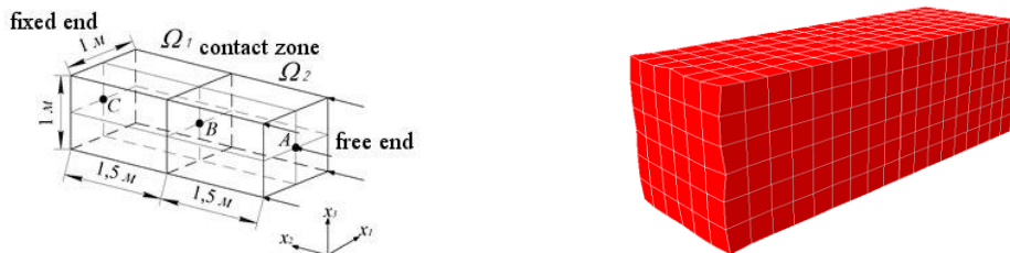
Fig. 2. Problem formulation (left) and boundary element mesh visualization (right).
