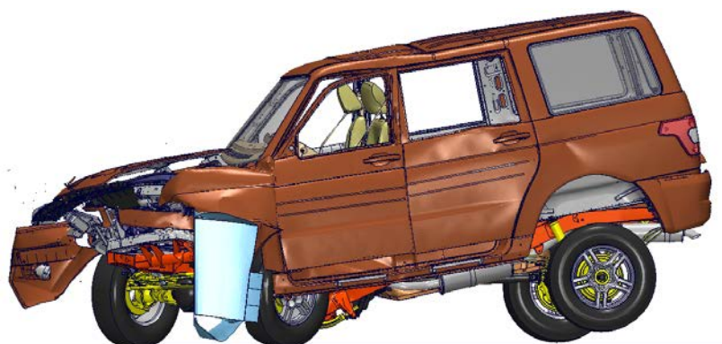
Fig. 11. Deformation with optimized material models.
