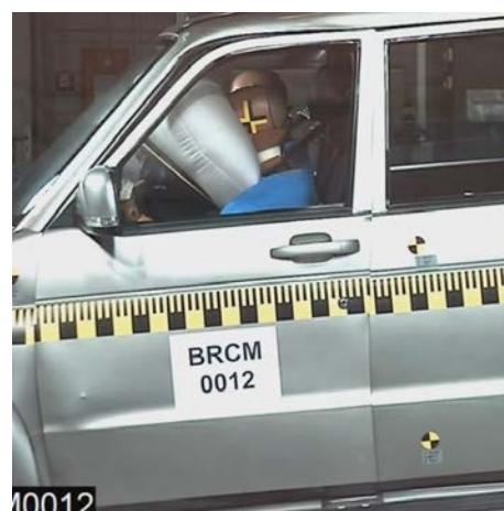
Fig. 17. Collision of dummy head with airbag, actual crash-test 90 ms.
