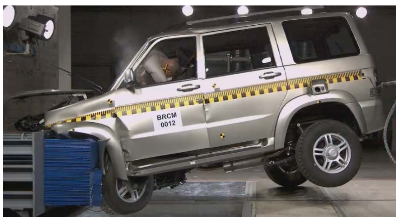
Fig. 12. Deformation in actual crash-test.
