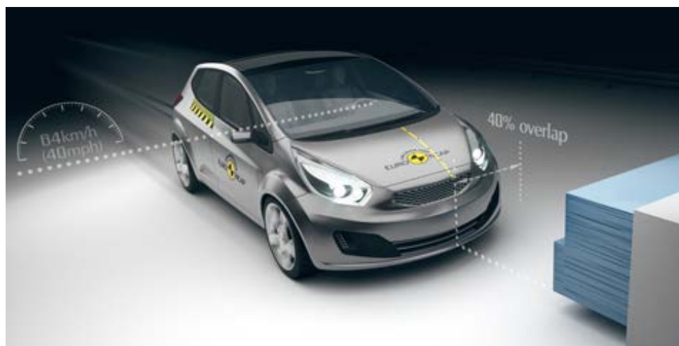
Fig. 1. Scheme of EuroNCAP frontal crash-test procedure.
