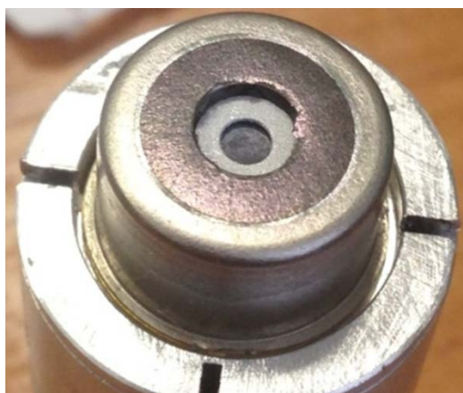
Fig. 12. Typical character of thin beryllium window fracture in the X-ray detector.
