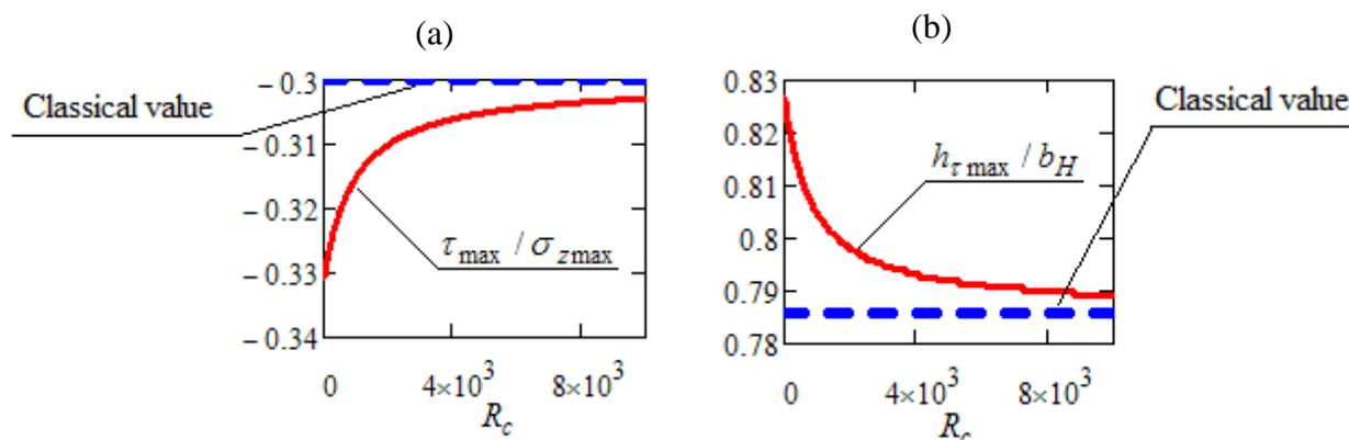
**Fig. 2.** Assessment results of the determination by using classical solutions for maximal shear stresses (a) and depth of its occurrence (b) according to the radius of the examined cylinder by using ACM-DS method.
