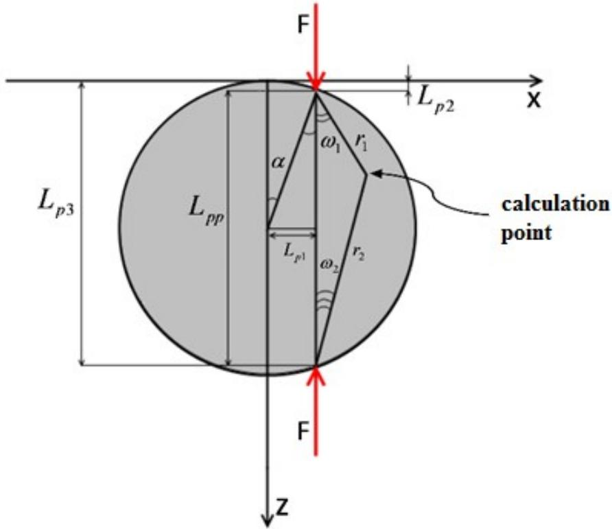
**Fig. 1.** Cylinder, compressed with opposite forces  $F$ , directed along axis  $Oz$ .
