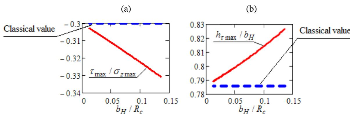
**Fig. 3.** Assessment results of the determination by using classical solutions of maximal shear stresses (a) and depth of its occurrence (b) according to the parameter  $b_H / R_c$  by using ACM-DS method.
