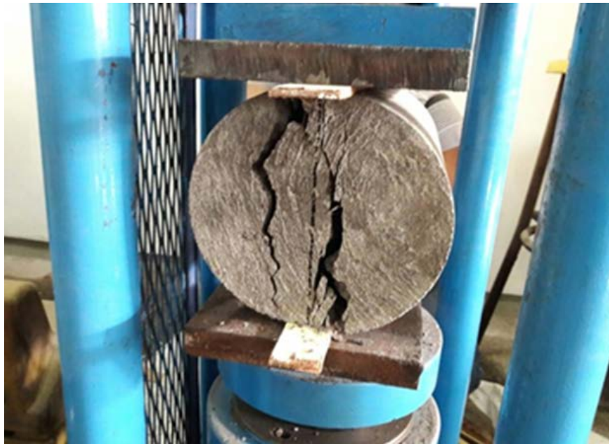
Fig. 4. Photo of testing concrete cylinder.
