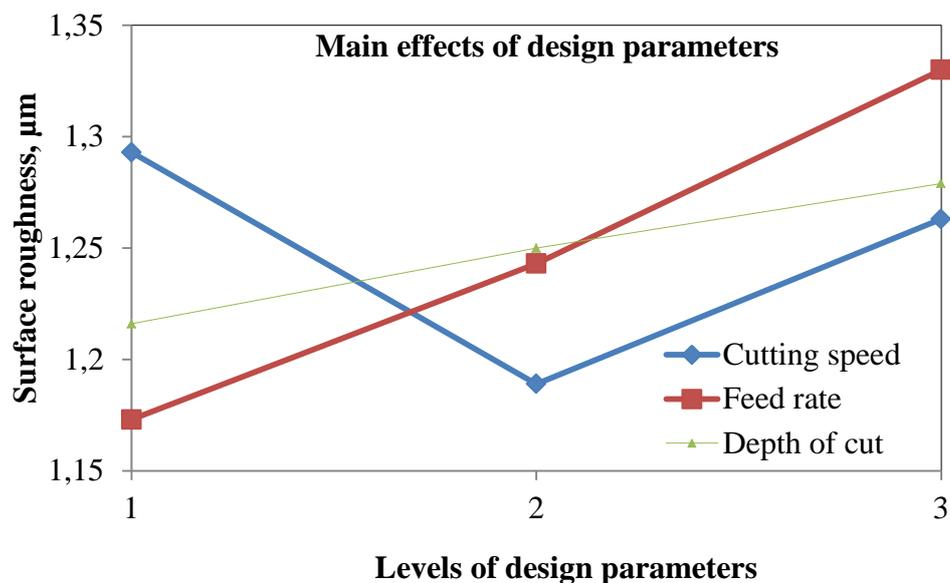
**Fig. 3.** Main effects of the design parameters on surface roughness during dry turning operation
