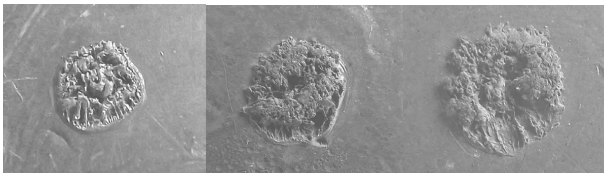
Fig. 2. Craters obtained in water after treating a lead sample by laser pulses with energy 10 J (a), 20 J (b), 40 J (c)
