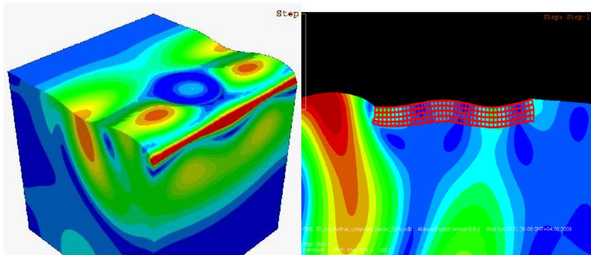
**Fig. 2.** Finite element model with a horizontal round-shaped barrier. 3D model (left) and cross section (right)
