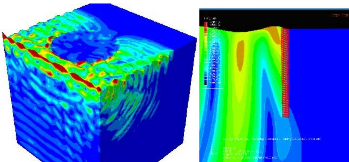
**Fig. 1.** Finite element model with a vertical round-shaped barrier. 3D model (left) and cross section (right)
