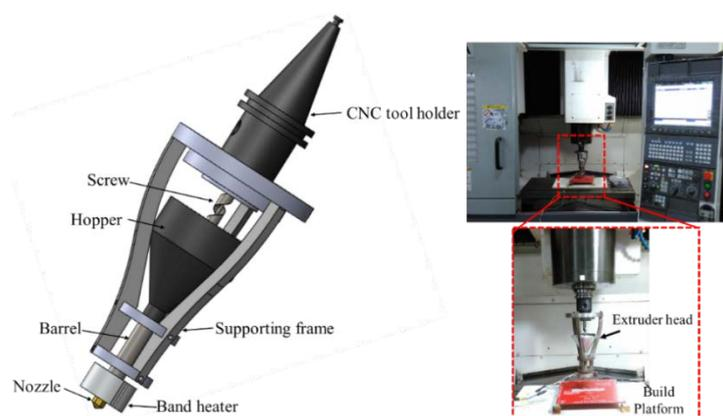
**Fig. 2.** Developed CNC assisted MDT system.
