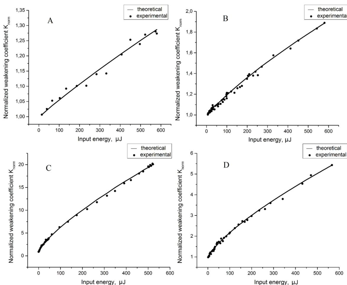
**Fig. 1.** Dependence of the normalized weakening coefficient on the input energy of the beam for aqueous solutions: (A) BSA (25 wt. %), (B) BC (2 wt. %), (C) BSA (25 wt. %) with SWCNT (0.3 wt. %), (D) BC (2 wt. %) with SWCNT (0.3 wt. %).
