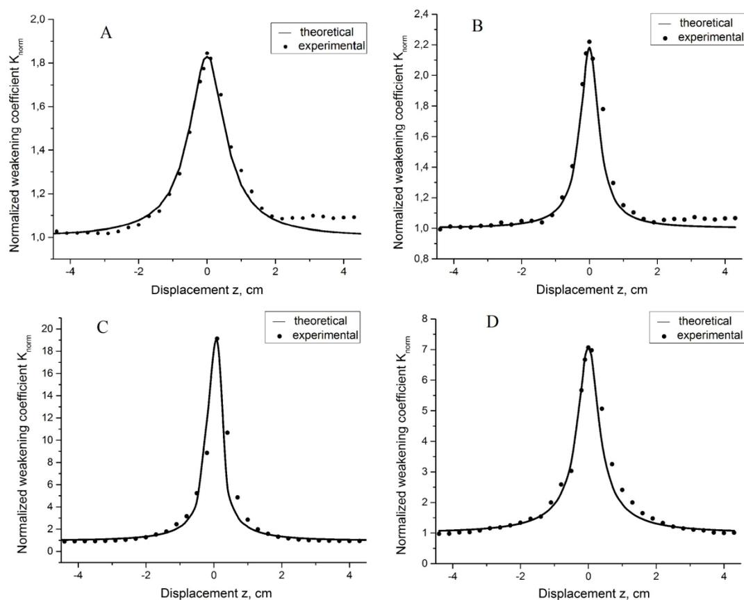
**Fig. 2.** Dependence of the normalized weakening coefficient on the position of the sample relative to the focus of the lens for aqueous solutions: (A) BSA (25 wt. %), (B) BC (2 wt. %), (C) BSA (25 wt. %) with SWCNT (0.3 wt. %), (D) BC (2 wt. %) with SWCNT (0.3 wt. %).
