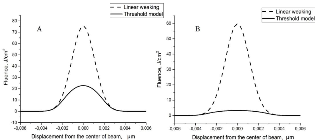
**Fig. 3.** Dependence of the light fluence distribution on the distance from the center of the beam for dispersions: (A) BC (2 wt. %), (B) BC (2 wt. %) with SWCNT (0.3 wt. %).
