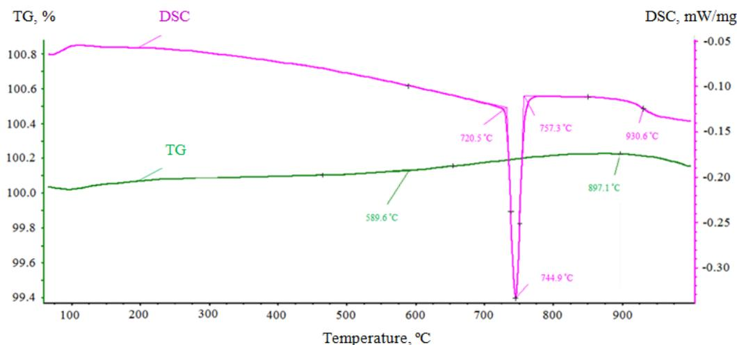
**Fig. 2.** Thermogram of eutectoid steel specimen continuous heating in argon
