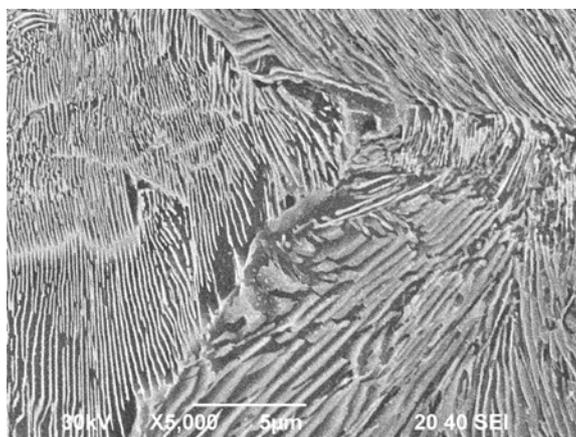
Fig. 1. Microstructure of high carbon steel 0.8 %C
