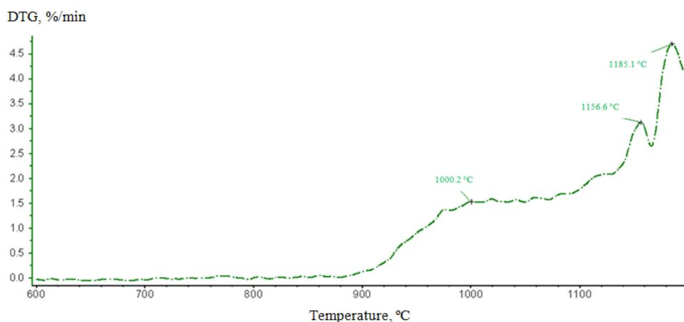
**Fig. 4.** Relationship between the eutectoid steel oxidation rate and temperature
