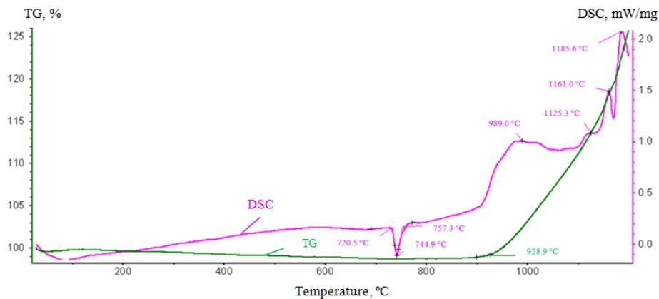
**Fig. 3.** Thermogram of steel grade 80 specimen continuous heating in air
