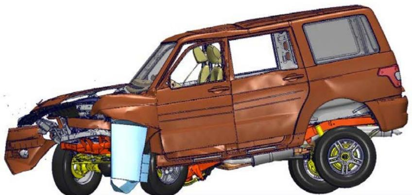
**Fig. 7.** Deformed SUV body FE model with calibrated GISSMO damage model defined
