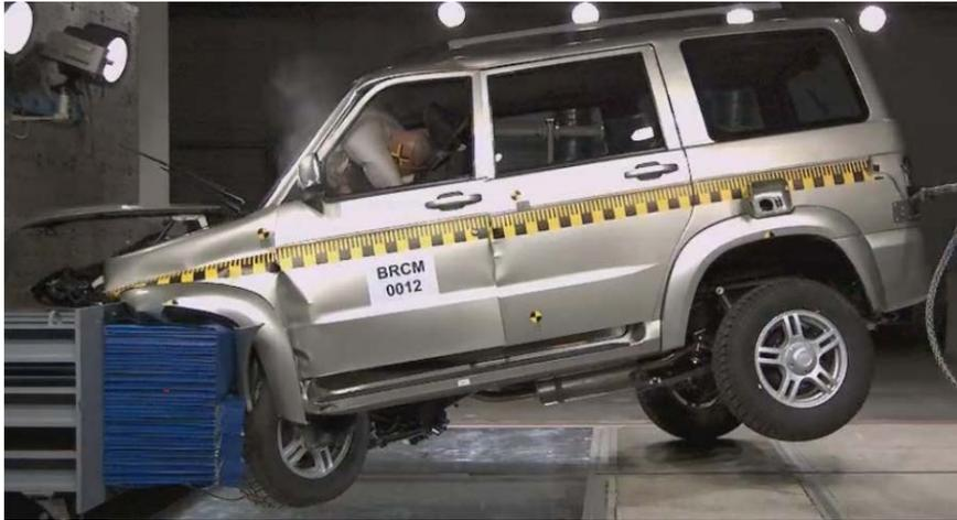
**Fig. 8.** Deformed SUV body, full-scale test
