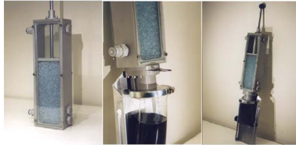
Fig. 18. The experimental cell for artificial porous medium
