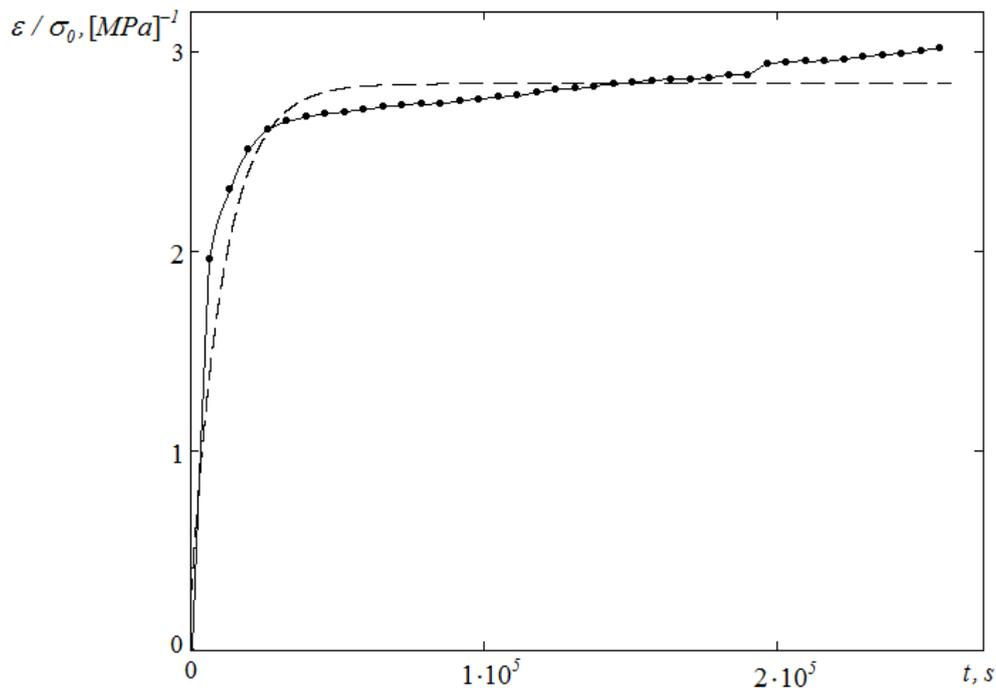
**Fig. 5.** The theoretical creep (compliance) curves according (5) and experimental points for polyurethane specimens tested on creep under constant load of 60 N and after aging according to program 3
