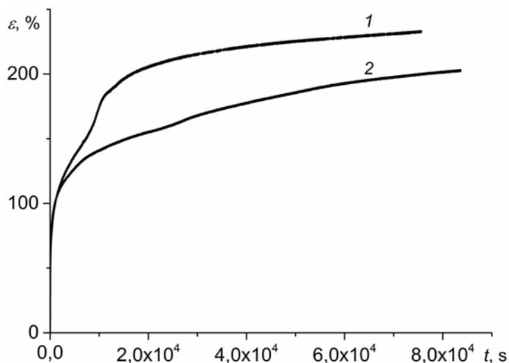
**Fig. 2.** Experimental creep curves under constant load of 70 N for polyurethane specimens without aging (curve 1) and after aging (curve 2)
