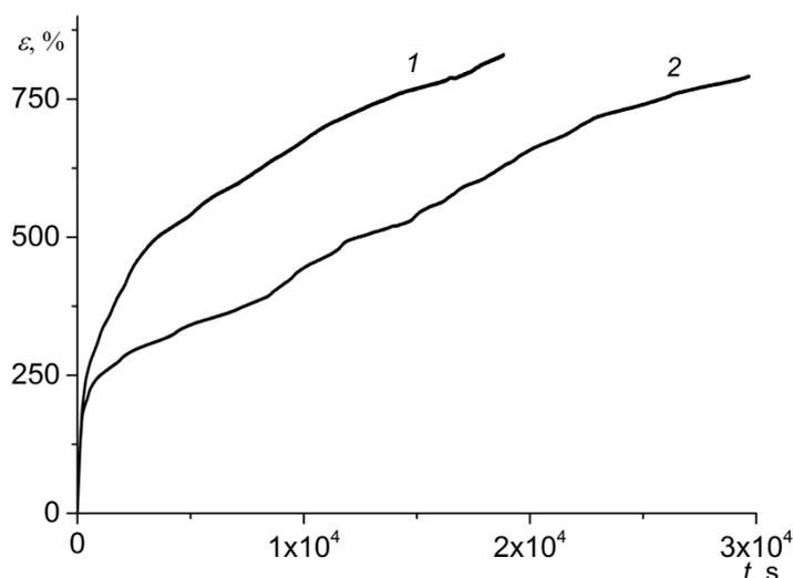
**Fig. 1.** Experimental creep curves under constant load of 80 N for polyurethane specimens without aging (curve 1) and after aging (curve 2)
