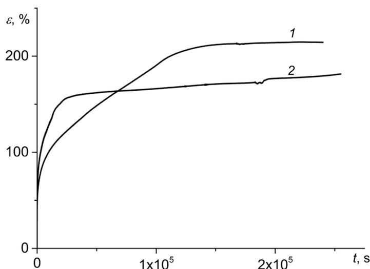
**Fig. 3.** Experimental creep curves under constant load of 60 N for polyurethane specimens without aging (curve 1) and after aging (curve 2)
