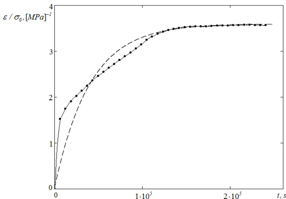
**Fig. 4.** The theoretical creep (compliance) curves according (5) and experimental points for polyurethane specimens tested on creep under constant load of 60 N without aging
