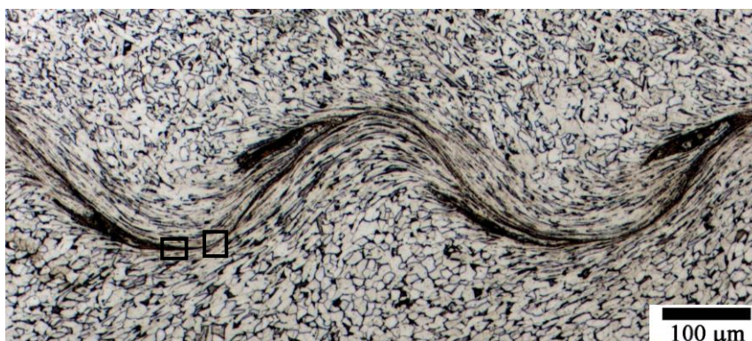
Fig. 1. General view of the wavy interface of the joint (the top plate is the flyer plate and the direction of detonation is from left to right). Rectangular frames indicate regions, from which specimens 1 (right) and specimen 2 (left) for microstructure investigation have been cut.
