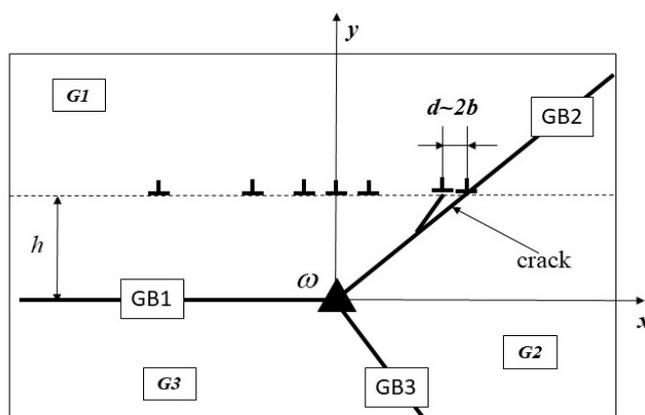
**Fig. 4.** Schematic plot of the crack nucleation at the head of edge dislocations pile-up.
