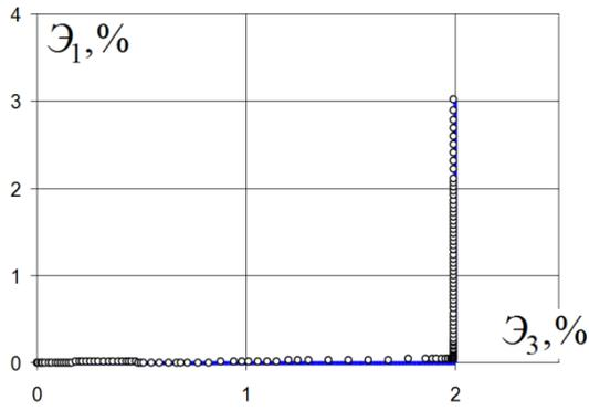
**Fig. 5.** Strain trajectory with the break angle  $90^\circ$
