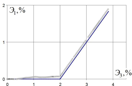
**Fig. 1.** Strain trajectory with the break angle  $45^\circ$
