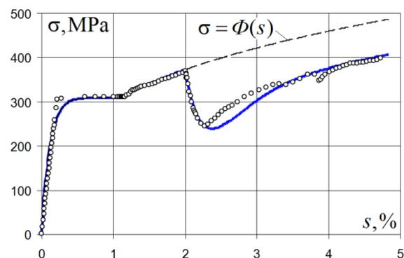
**Fig. 11.** Chart of deformation  $\sigma - s$
