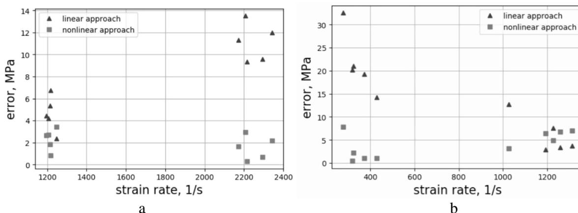
**Fig. 8.** Model identification approaches comparison: a – lime-sand brick ( $\sigma_c = 13.1$  MPa,  $\tau = 28$   $\mu\text{s}$  - nonlinear approach,  $\tau = 11,3$   $\mu\text{s}$  - linear approach), b – ceramic brick ( $\sigma_c = 13.7$  MPa,  $\tau = 49$   $\mu\text{s}$  - nonlinear approach,  $\tau = 17,9$   $\mu\text{s}$  - linear approach)
