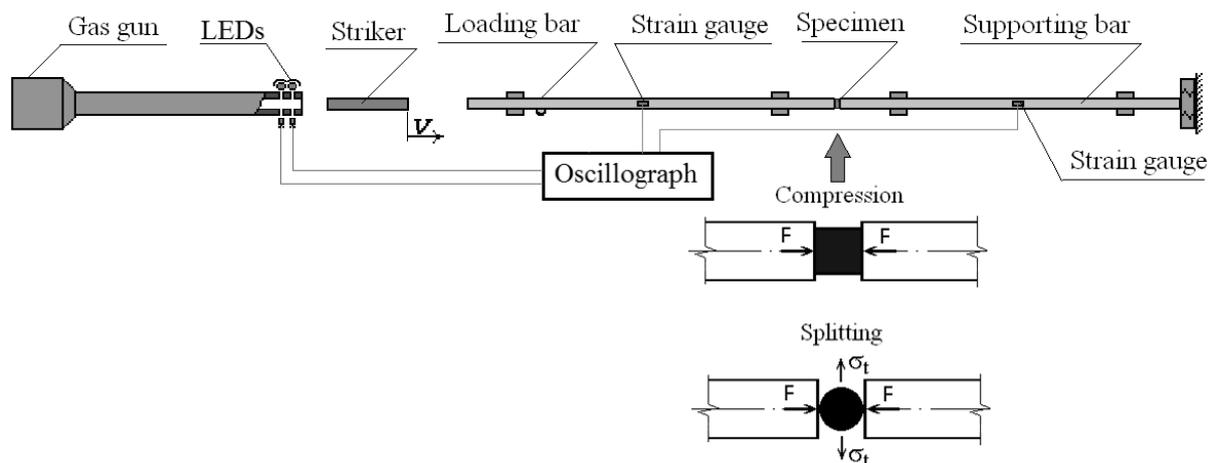
**Fig. 1.** Methods used in dynamic testing of ceramic and lime-sand bricks
