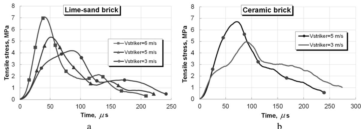
Fig. 4. Deformation diagrams of samples of sand-lime (a) and ceramic (b) brick at splitting
