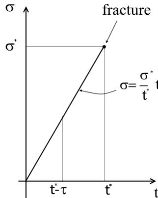
Fig. 6. Linear approach to criterion identification
