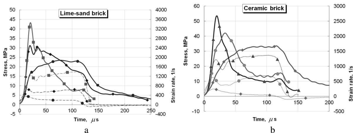
**Fig. 2.** Deformation diagrams of samples of lime-sand (a) and ceramic (b) brick at compression
