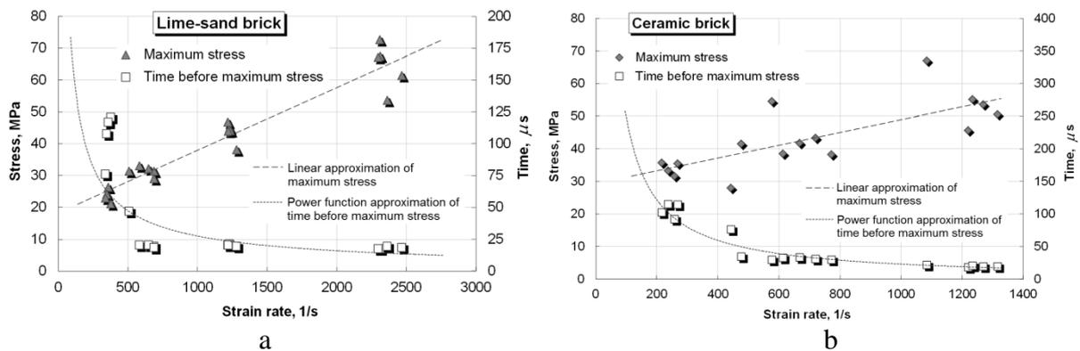
**Fig. 3.** Dependencies of mechanical properties versus the strain rate for lime-sand (a) and ceramic (b) bricks at compression
