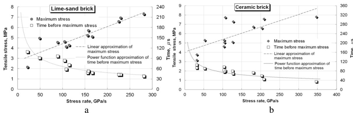
Fig. 5. Dependencies of mechanical properties versus the stress rate lime-sand (a) and ceramic (b) bricks at splitting
